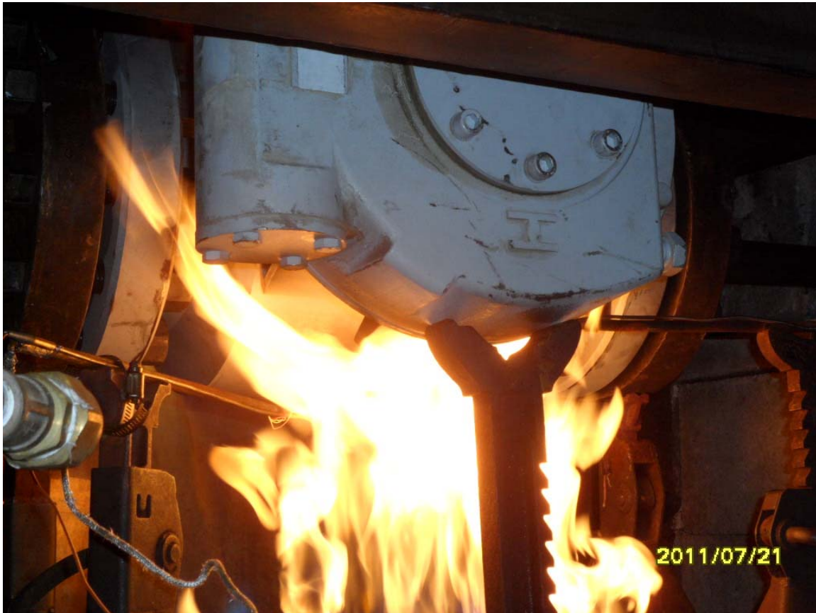
Valve During Burn (Torches not fully on)
