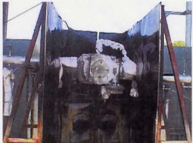
Valve After Burn and Cool Down
