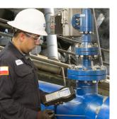
Unlike other testing methods that require the removal of large amounts of insulation, ValvTechnologies requires only small drill holes for access with a 3/8" diameter transducer.
