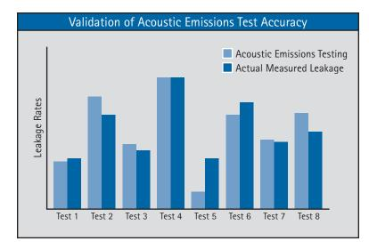
Referring to the table, the process has been third-party verified for accuracy. On populations of valves, the process has demonstrated to be within 4% of the laboratory verified leakage rate and within 10% over two standard deviations.
