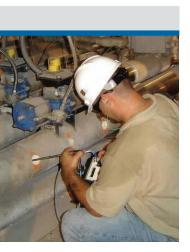
Unlike other testing methods that require the removal of large amounts of insulation, ValvTechnologies requires only small drill holes for access with a 3/8 inch diameter transducer.
