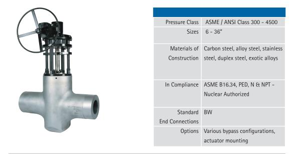
Receive in-line valve repairability in large-diameter, high-energy piping systems with the ValvTechnologies' PSG series. Proven precisely right for steam and feedwater applications, the PSG series offers our rigorous four-year guarantee against leakage and low-cost maintain-ability.
