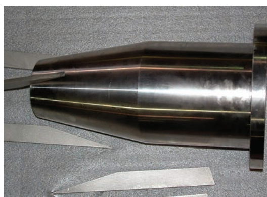
Pictured left: is a 10" diameter, de-coke t-section. The overlay is 200 degree grid, .350 thick.
