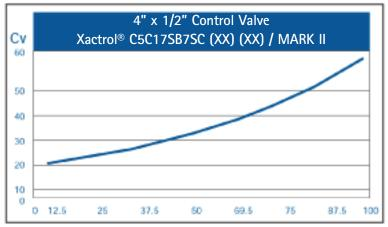
Each valve package will come complete with its own flow test curve to ensure complete reliability. The above graph is from an actual flow loop test as supplied to the customer.
