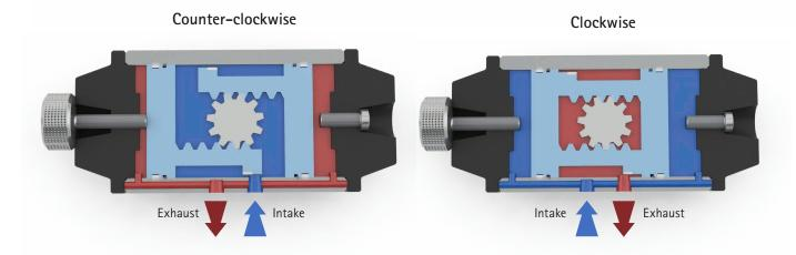
Counter clockwise output operation is achieved by inserting pressure into the intake to force the pistons apart thus rotating the actuator pinion counter clockwise. During the operation, air from the outer chambers is exhausted. Clockwise output operation is achieved by reverse of the above.
