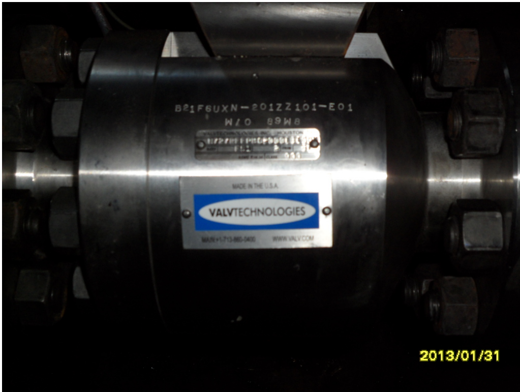
Test Valve Prior to Burn
