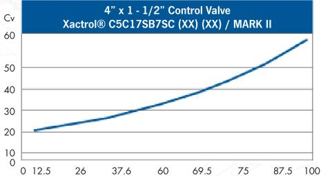
Each valve package will come complete with its own flow test curve to ensure complete reliability. The above graph is from an actual flow loop test as supplied to the customer.
