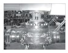
This NexTech® 20" valve was part of a HIPPS skid, supplied to the Pacific Rim. The valve was rigorously tested to meet ValvTechnologies' zero-leakage test standard, as well as SIL 3 requirements.
