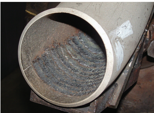
10" diameter, de-coke t-section. The overlay is 200° grid, .350 thick.
