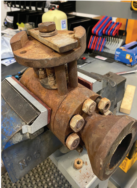
ValvTechnologies' boiler drum vent valve after 24 years in service.
