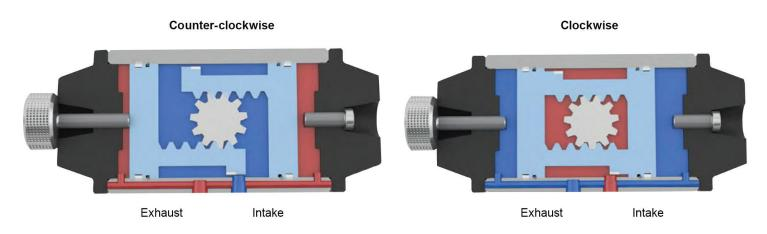
Counter clockwise output operation is achieved by inserting pressure into the intake to force the pistons apart thus rotating the actuator pinion counter clockwise. During the operation, air from the outer chambers is exhausted. Clockwise output operation is achieved by reverse of the above.
