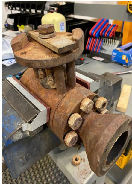
ValvTechnologies' boiler drum vent valve after 24 years in service.
